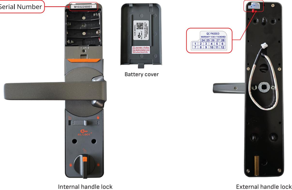
2. Removing the red-colored connector from the circuit board will immediately void the warranty (see the attached image).
